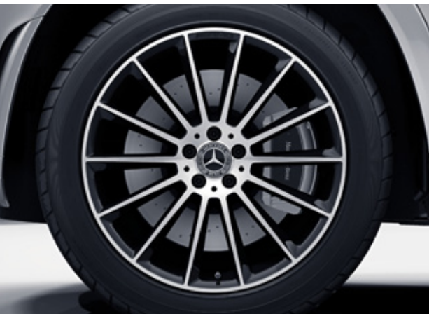
RWB 21" AMG alloy wheels (4) – multi-spoke light-alloy wheels painted in black with a high-sheen finish, front 275/45 tyres; rear: 315/40 tyres
