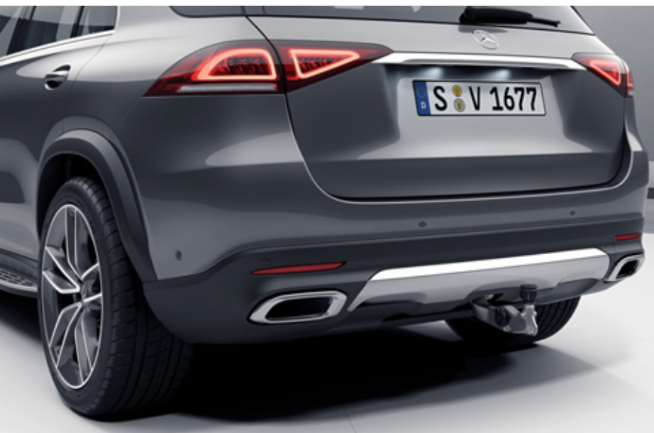
Electronically-folding tow bar (includes 13-pin socket; ESC)
