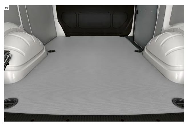
**04 Universal floor (for fittings).** The ideal preparation for subsequent installation of cabinet systems from various manufacturers<sup>3</sup>. Special adapters<sup>4</sup> in the recesses in the floor covering permit flexible installation of cabinet systems at any time without gluing or drilling. Subsequent removal of the floor leaves only minimum traces. Optional on panel van models. | S | H |
