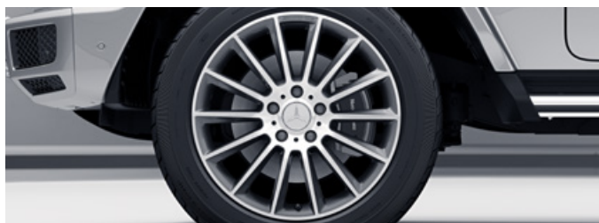
RK4 20" AMG alloy wheels - multi-spoke design, painted titanium grey with a high-sheen finish, 275/50 R20 tyres
