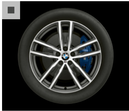
19" M light alloy Double-spoke style 698 M wheels, Bicolour Ferric Grey, 7.5J x 19 with 245/50 R19 non run-flat tyres. Standard for M Sport and M Sport X models.
