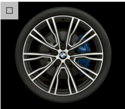
21" BMW Individual light alloy V-spoke style 726 wheels, Bicolour Orbit Grey, front 8.5J x 21 with 245/40 R21, rear 9.5J x 21 with 275/35 R21 run-flat tyres. Optional for M Sport and M Sport X models.
