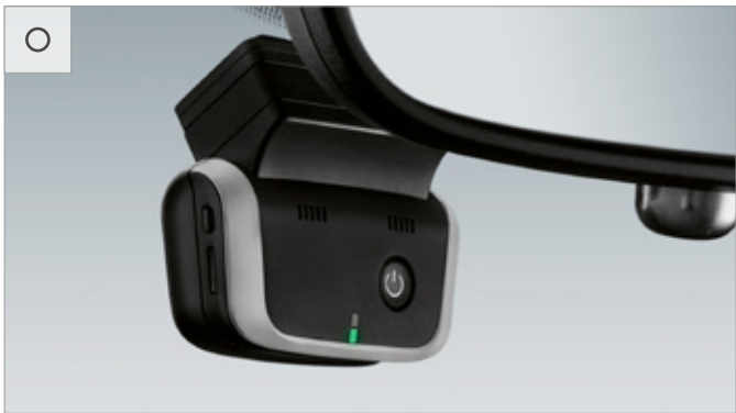
The BMW Advanced Car Eye is a highly sensitive full-HD camera that captures situations in front of and behind the car, even when it is parked. In the event of disturbances outside the vehicle, the camera automatically records the occurrence in order to document possible accidents.
