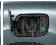
Charge Complete Mode (Constant green LED)
