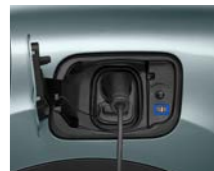
Deferred Charge Mode (Flashing blue LED)
