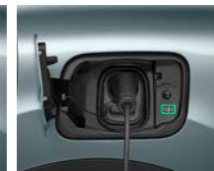
Charging Mode in Progress (Flashing green LED)
