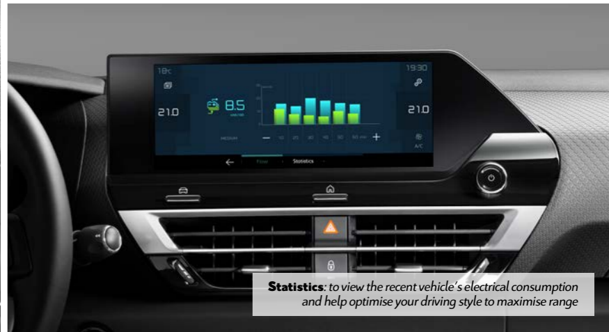
Instrument panel including the essential information relating to the electrical system
