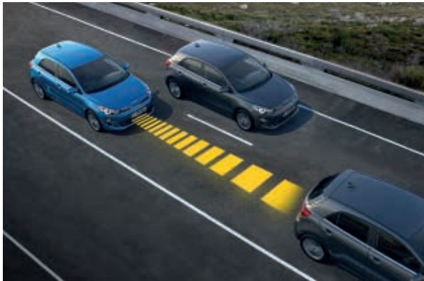
Forward Collision-Avoidance Assist. This system looks out for possible collisions with pedestrians, cyclists and other cars. It warns you and helps you brake if you aren't reacting fast enough.
