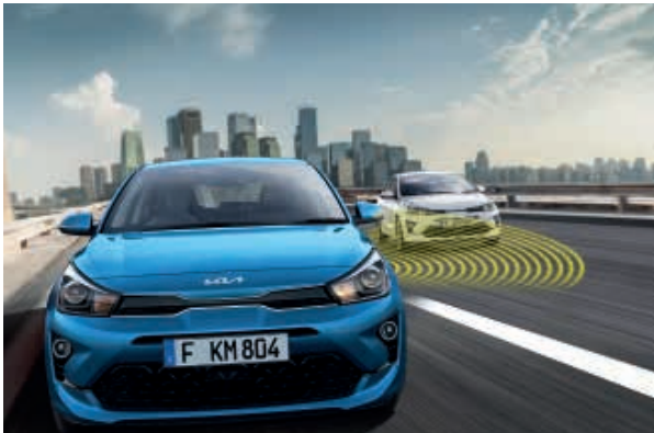
Blind-Spot Collision Warning. This system continuously monitors your blind spot and vehicles attempting to overtake you. A warning symbol lights up in your door mirror if a vehicle is detected, and an audible alert sounds if you indicate despite the obstacle. The system might even interact with your steering if it senses a high risk of collision (grade dependent).
