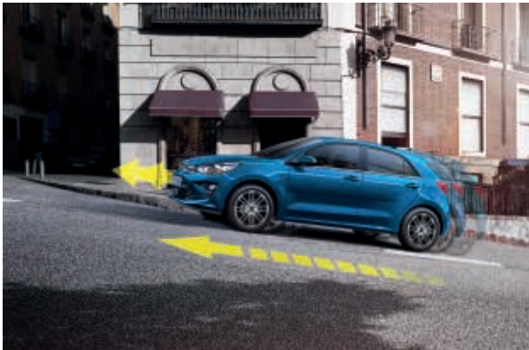
Hill Start Assist Control. Get added support for those tricky hill starts. Hill Start Assist Control prevents you from rolling backwards when you remove your foot from the brake.
