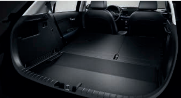
Adjustable cargo floor. Position the cargo-area floor higher to be flush with the folded seat backs (left), or lower to accommodate tall items (right). (The cargo floor in Mild Hybrid versions is always positioned lower.)
