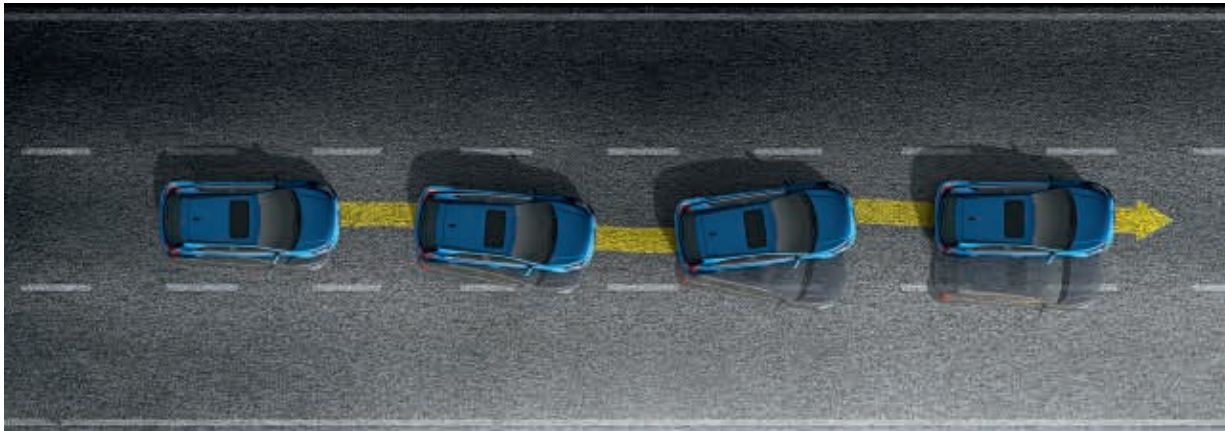
Straight-Line Stability. When braking in a straight path, this system senses any difference in applied brake pressure between the right and left wheels, and adjusts the pressure to counteract yaw and maintain straight-line stability.
