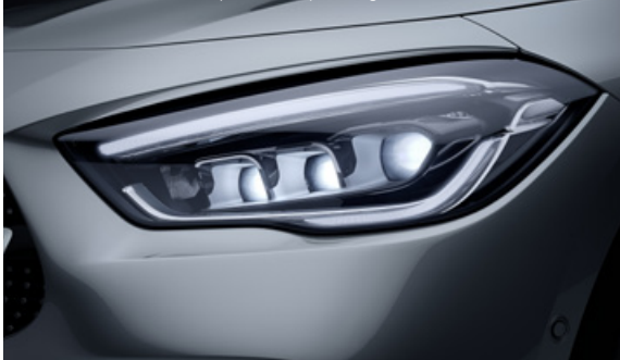
MULTIBEAM LED headlamps with Adaptive Highbeam Assist
