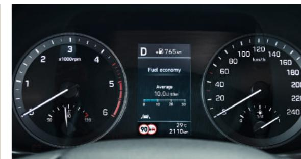
**Intelligent Speed Limit Warning (ISLW)\*:** Recognizes road speed signs and displays the speed limit in real time in both the navigation system display and instrument cluster.
