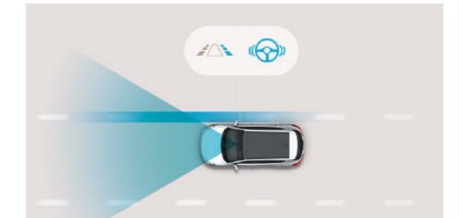
**Lane Keeping Assist:** The Lane Keeping Assist (LKA) uses the front multi-function camera to monitor the lines of the road. In case of an unintended lane departure, it warns you and can apply counter steering torque to guide the car back to the lane.
