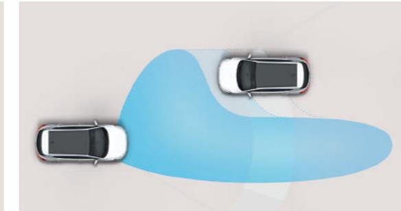
**High Beam Assist (HBA):** Less stress and maximum visibility. HBA not only detects oncoming vehicles but also vehicles in the same lane ahead and switches to low-beam as appropriate.
