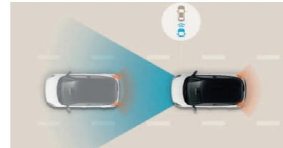
**Forward Collision-Avoidance Assist (FCA):** Sensing the road ahead with the multi-function camera, FCA warns you and then automatically brakes when it detects sudden braking by a car ahead. Includes pedestrian detection.
