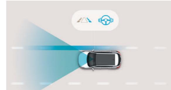
**Lane Keeping Assist:** The Lane Keeping Assist (LKA) uses the front multi-function camera to monitor the lines of the road. In case of an unintended lane departure, it warns you and can apply counter steering torque to guide the car back to the lane.
