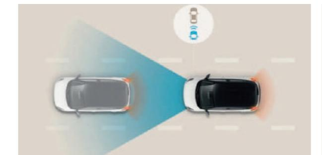
**Forward Collision-Avoidance Assist (FCA):** Sensing the road ahead with the multi-function camera, FCA warns you and then automatically brakes when it detects sudden braking by a car ahead. Includes pedestrian detection.
