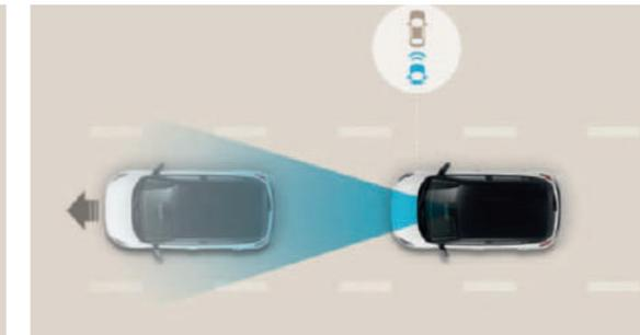
**Leading Vehicle Departure Alert (LVDA):** This clever feature for city driving alerts the driver when the vehicle in front departs from an idle state, like at a stoplight or in a traffic jam.
