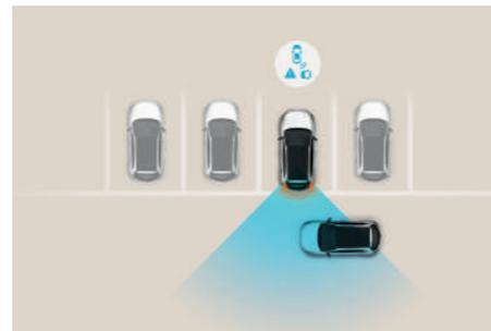
**Rear Cross-traffic Collision Warning (RCCW):** Sensors detect vehicles approaching from both sides when the New i30 is in reverse, avoiding collisions in congested or reduced visibility environments such as car parks.
