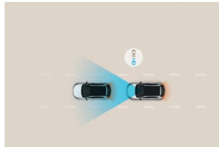
**Front Collision Avoidance (FCA):** The front view camera and radar sensors warn drivers of imminent collisions with vehicles and objects, applying the brakes when necessary to avoid collisions.
