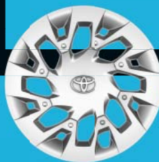
15" steel wheels with wheel caps (8-double-spoke) Standard on x-play
