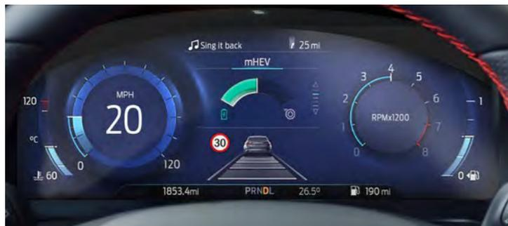
Fiesta EcoBoost Hybrid displays how much electrical power has been generated by the mild-hybrid system, and tracks whether energy is currently being returned to the battery or used to assist fuel efficiency or performance.
