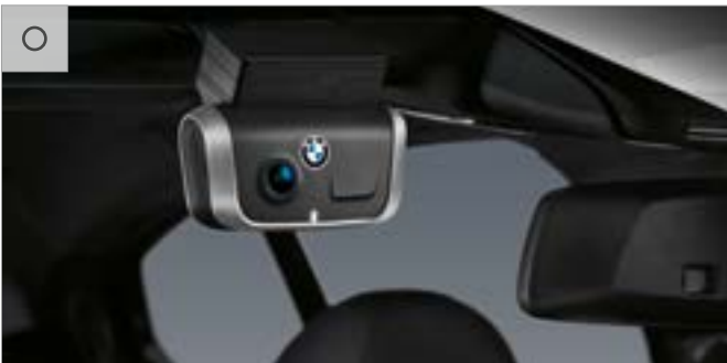
BMW Advanced Car Eye 2.0 is a highly sensitive full HD camera, which automatically records what is going on around the vehicle during disturbances and driving situations.
