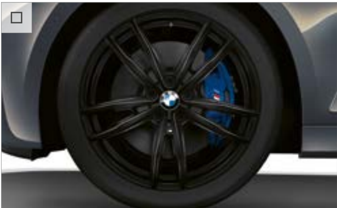
19" M light alloy Double-spoke style 791 M wheels, Jet Black, front 8 J x 19 with 225/40 R19 run-flat tyres, rear 8.5 J x 19 with 255/35 R19 run-flat tyres. Standard for M Sport Plus Edition models. Only available as part of Shadowline Plus Package on M340i xDrive and M340d xDrive models.
