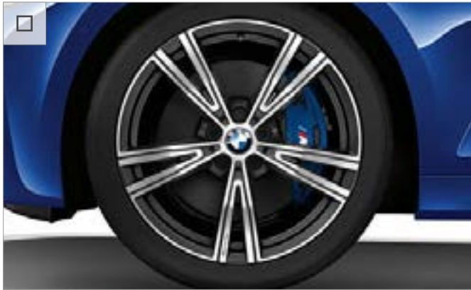
19" BMW Individual light alloy Double-spoke style 793 wheels, Bicolour Orbit Grey, front 8 J x 19 with 225/40 R19 run-flat tyres, rear 8.5 J x 19 with 255/35 R19 run-flat tyres. Optional for Sport and M Sport models. Not available with the M Sport Plus Package.
