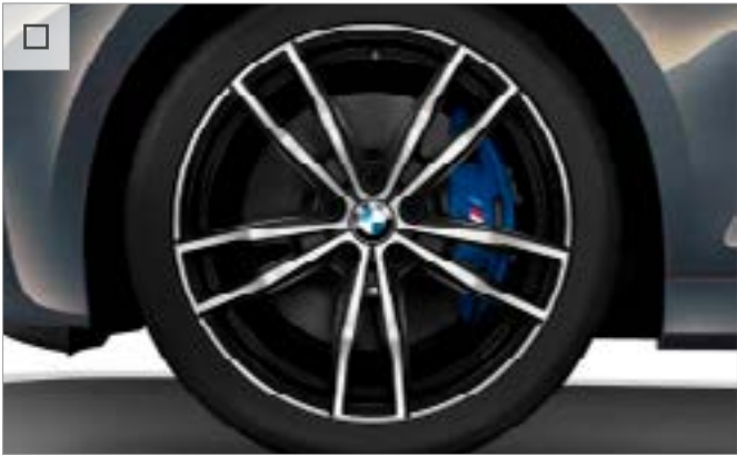
19" M light alloy Double-spoke style 791 M wheels, Bicolour Jet Black, front 8 J x 19 with 225/40 R 19, rear 8.5 J x 19 255/35 R 19 run-flat tyres. Optional for M Sport and M Sport Plus Edition models. Only in combination with the M Sport Plus Package.
