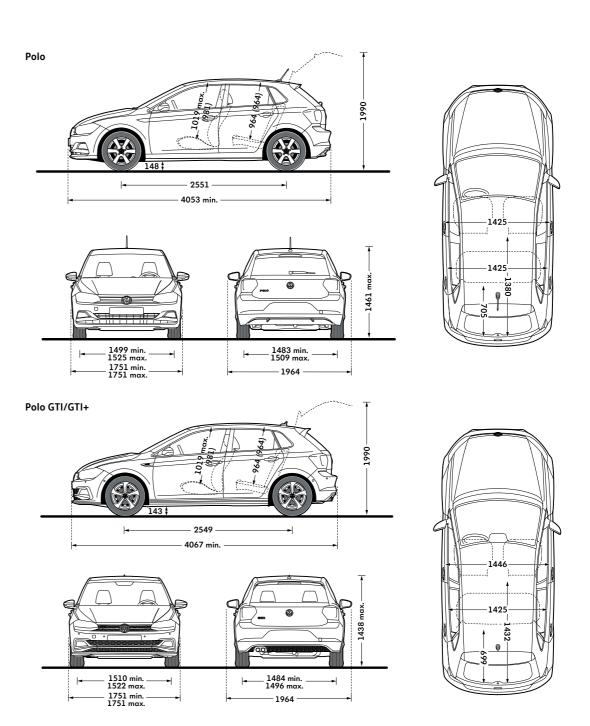
All figures in millimetres. On illustrations, where arrows and figures are shown inside of the vehicle, the measurements are for interior dimensions. Where arrows and figures are shown outside of the vehicle, the measurements are for exterior dimensions.
