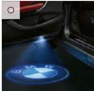
When the doors are opened, the LED Door Projectors project one of a choice of four graphics on the ground adjacent to the vehicle, for perfect illumination of the entry area.
