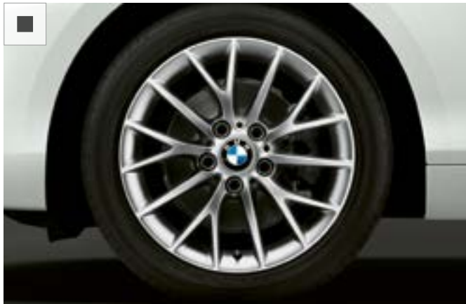
17" light alloy Y-spoke style 380 wheels, Reflex Silver, 7J x 17 with 205/50 R17 run-flat tyres. Standard for SE models.
