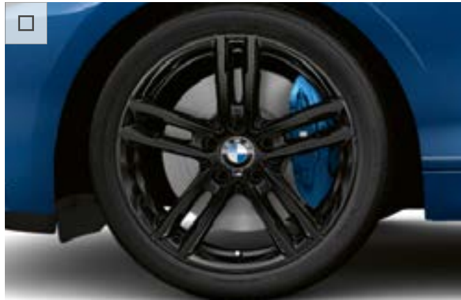
18" M light alloy wheels Double-spoke style 719 M, Jet Black, front 7.5J x 18 with 225/40 R18, rear 8J x 18 with 245/35 R18 run-flat tyres for M Sport models / non-run flat tyres for M240i models. Optional for M Sport and M240i models.
