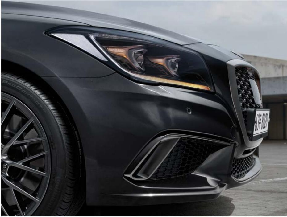
**Sequential turn signals & Full LED adaptive headlamps** \_ Turn signals light up sequentially and headlamps feature prominent copper chrome details. Vertical air curtains below headlamps improve aerodynamic and brake-cooling performance.
