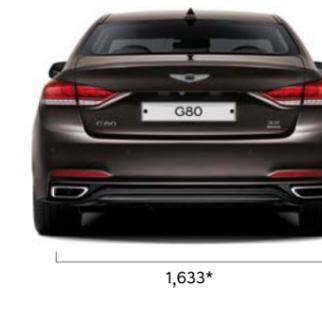
Units: mm, \* based on 245/40R19 tires in the front and 275/35R19 tires in the back
