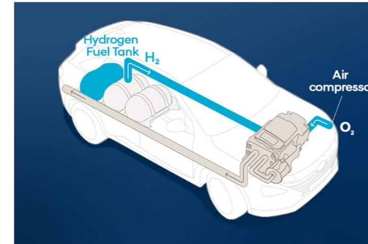
Hydrogen from the fuel tank is fed to the fuel cell stack, where it is mixed with clean, compressed air.
