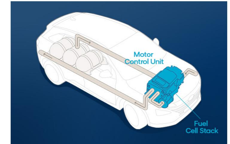
The Hydrogen reacts with Oxygen in the fuel cells, generating electricity and water.
