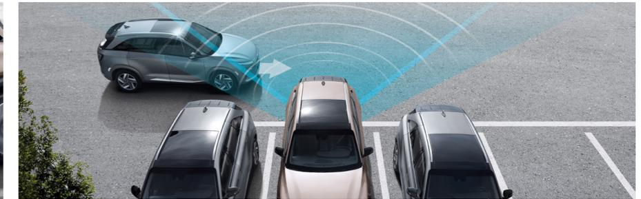
**Rear Cross-Traffic Collision-Avoidance Assist (RCCA):** Radar sensors in the rear bumper monitor cross traffic approaching from left and right side of the vehicle during reverse manoeuvres, and if necessary apply emergency braking to prevent collision.
