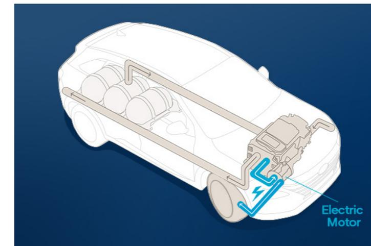
The electricity is supplied to the electric motor and to the high voltage battery to power the vehicle.
