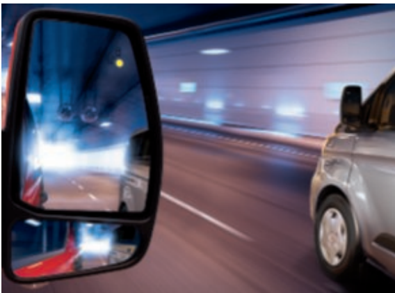
Blind Spot Information System As another vehicle – a car, van or lorry – enters your blind spot whilst travelling, the system is designed to alert you with a warning light clearly displayed in the corresponding door mirror.
