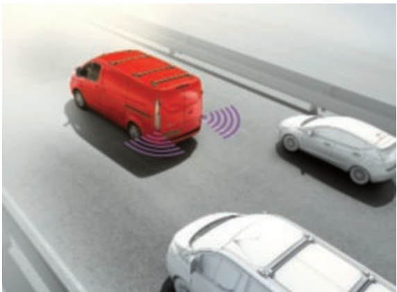
Blind Spot Information System As another vehicle – a car, van or lorry – enters your blind spot whilst travelling, the system is designed to alert you with a warning light clearly displayed in the corresponding door mirror.
