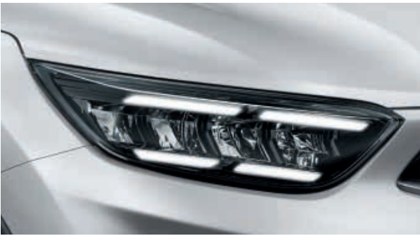
LED projection headlamps. The full LED headlamps produce a more powerful and precise light, allowing you to better detect obstacles at night (grade dependent).
